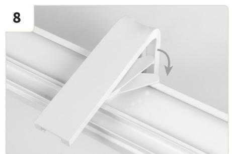
Begin with the installation of the leftmost track rail. The lever is oriented towards the wall. Lift the track to the ceiling so that the fixture sits in the groove on the upper side of the rail. Turn the lever until the track rail is secured.
